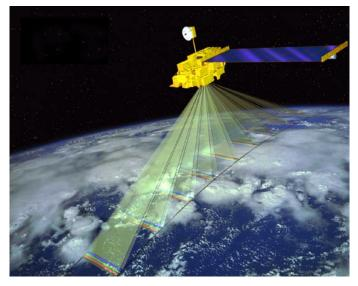
The MISR instrument on the Terra satellite views the atmosphere and Earth's surface from nine different angles.
