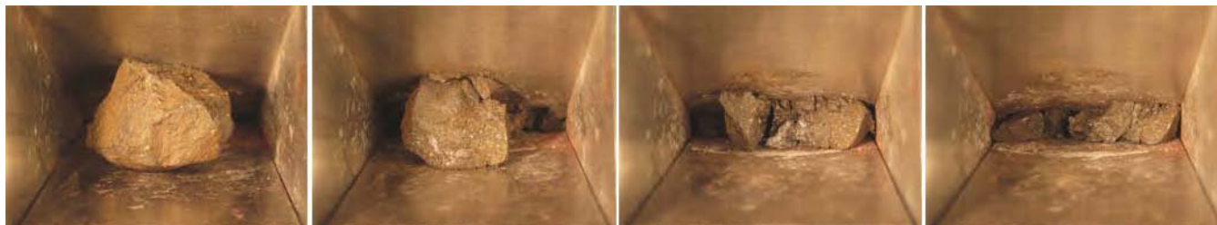
Looking down on the jaws of the Mars Rock Crusher, we see a magnetite rock get crushed into smaller and smaller particles.
