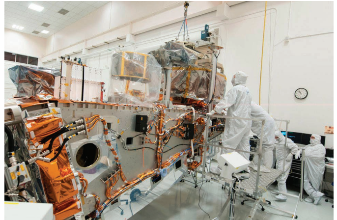
Image Caption: Ball and Raytheon technicians integrate the VIIRS Optical and Electrical Modules onto the JPSS-1 spacecraft in 2015. The spacecraft will be ready for launch later this year. Image Credit: Ball Aerospace & Technologies Corp.
