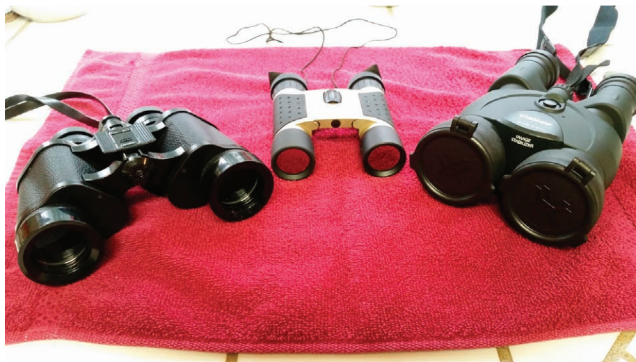
Image Caption: Bushnell 7x35mm widefield binoculars, Coronado 10x25mm binoculars with built-in white light solar filters, and Canon 12x36mm image stabilized binoculars. Credit: Ken Sperber
